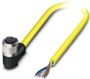
Sensor/actuator cable, 5-position, PVC, yellow, free cable end, on Socket angled M12 SPEEDCON, A-coded, cable length: 2 m
