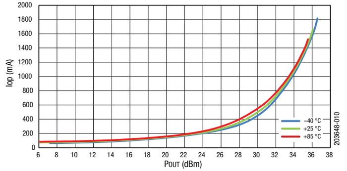
**Figure 10. Operating Current vs POUT Across Temperature**
