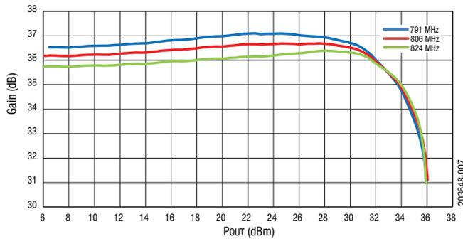
Figure 7. Gain vs POUT Across Frequency
