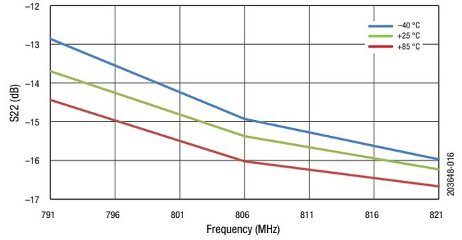
**Figure 16. Output Return Loss vs Frequency Across Temperature**
