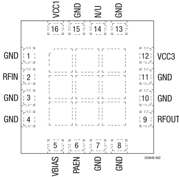
Figure 2. SKY66289-11 Pinout (Top View)
