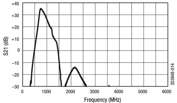
**Figure 14. Wide Band Small Signal Gain vs Frequency**
