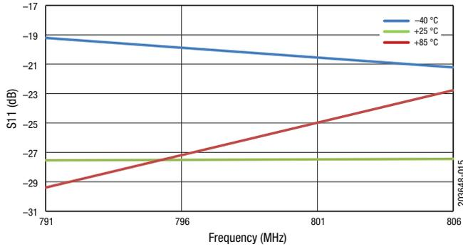
**Figure 15. Input Return Loss vs Frequency Across Temperature**
