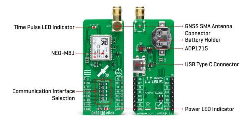
For even better and faster positioning improvement, the NEO-M8J supports the augmentation of QZSS, GAGAN, and IMES together with WAAS, EGNOS, and MSAS. The future-proof NEO-M8I includes an internal Flash that allows future firmware updates, making it ideally suited to industrial and automotive applications. It also supports message integrity protection, geofencing, and spoofing detection with configurable interface settings to fit customer applications easily.
