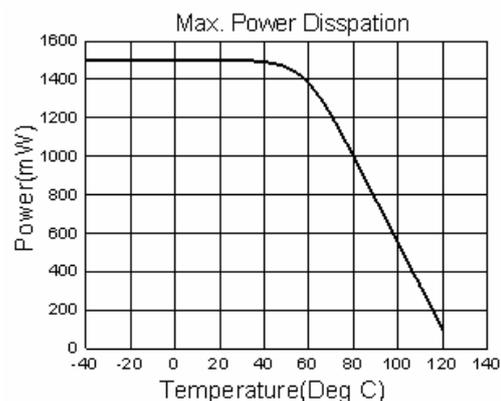
Note that the device power dissipation will most often be a maximum at minimum supply voltage. It will also increase if the efficiency of the circuit is low. This may result from the use of unsuitable coils, or excessive parasitic output capacitance on the switch output. When the application is limited by the internal power dissipation of the device, the ESOP8 package is recommended because of its enhanced power dissipation ability.
