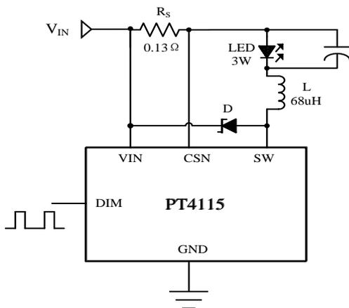
A value of 1uF will reduce the supply ripple current by a factor three (approx.). Proportionally lower ripple can be achieved with higher capacitor values. Note that the capacitor will not affect operating frequency or efficiency, but it will increase start-up delay and reduce the frequency of dimming, by reducing the rate of rise of LED voltage.
