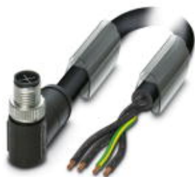
Power cable, 4-position, PUR halogen-free, black-gray RAL 7021, Plug angled M12 SPEEDCON, S-coded, on free cable end, cable length: 15 m, for AC current up to 12 A/630 V
