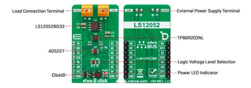
The eFuse uses the <u>TP86R203N</u>L, an N-channel MOS from Toshiba, as a gate to the output screw terminal. The current limit on this eFuse 7 Click can be programmed. For this purpose, there is the AD5227, a 64-position up/down control digital potentiometer from Analog Devices. This 10K end-to-end potentiometer, in variable resistor configuration, is used to feed the current limit program pin of the eFuse.
