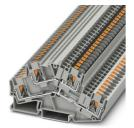
Double-level terminal block, with equipotential bonder, nom. voltage: 800 V, nominal current: 28 A, connection method: Push-in connection, 1st and 2nd level, cross section:  $0.2~\text{mm}^2$  -  $6~\text{mm}^2$ , mounting type: NS 35/7,5, NS 35/15, color: gray
