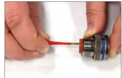
Plastic tool with contact in proper position.
