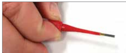
Plastic tool with contact in proper position.
