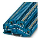
Double-level terminal block, nom. voltage: 800 V, nominal current: 28 A, connection method: Push-in connection, 1st and 2nd level, cross section:  $0.2~\text{mm}^2$  -  $6~\text{mm}^2$ , mounting type: NS 35/7,5, NS 35/15, color: blue
