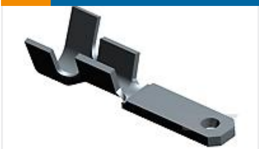
TE Part #63138-1 110 FASTON REC 22-18 AWG TPBR
