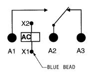
**NOTE:** Polarity must be observed with DC coil supply. Relay is polarized with a permanent magnet and will not operate or be damaged by reverse polarity.
