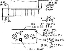
All Enclosures have cupro-Nickel cans bright acid tin/lead plated after assembly to terminal headers.
