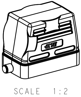
TYPE-5:H10B HOOD,LOW CONSTRUCTION, NO ENTRY,2 EAR OTHER SPEC REFER TO TYPE-1 类型-5:H10B上壳,低结构,无出线孔,2耳 其它规格尺寸参照类型-1
