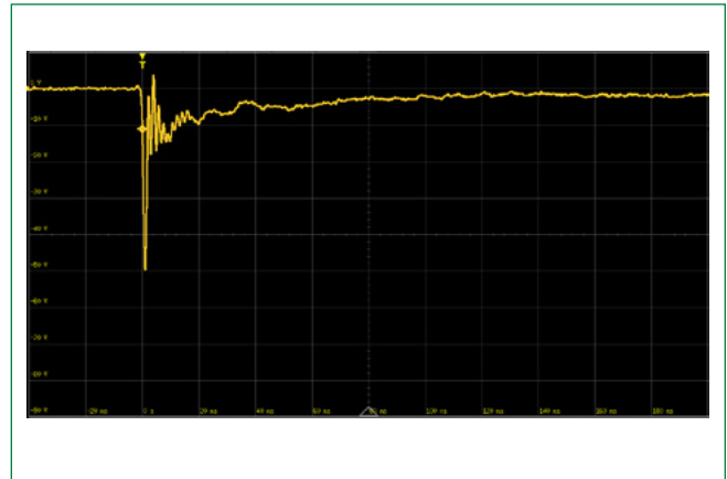
IEC 61000-4-2 -8 kV Contact ESD Clamping Voltage
