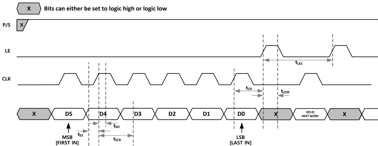
The BDA4601 has a 3-wire serial peripheral interface (SPI): serial data input (SERIN), clock (CLK), and latch enable (LE). The serial control interface is activated when P/S is set to HIGH.
