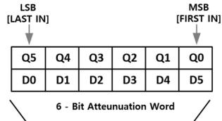
The attenuation word is derived directly from the value of the attenuation state. To find the attenuation word, multiply the value of the state by four, then convert to binary.
