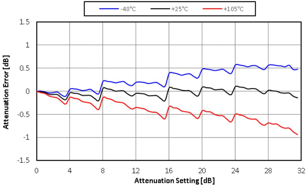
Figure 17. Attenuation Error @3500MHz vs Temperature
