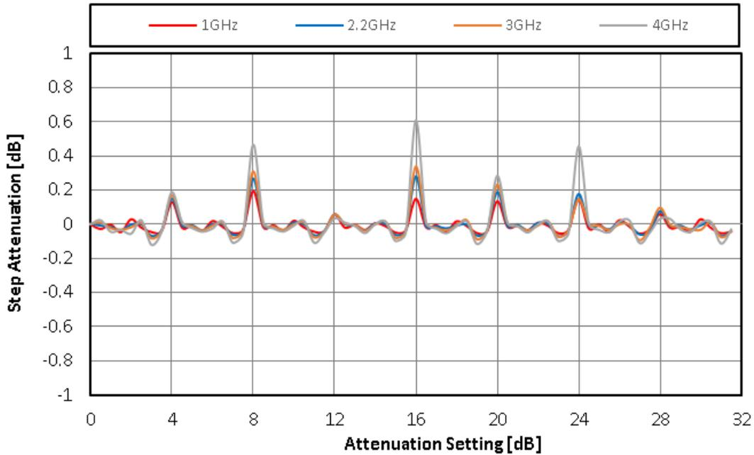
Figure 24. 0.5dB Step Attenuation vs Frequency
