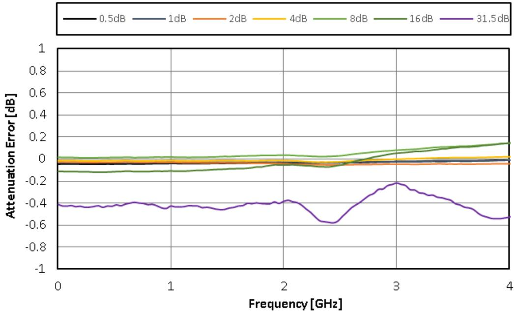
Figure 26. 0.5dB Major Attenuation Error vs Frequency
