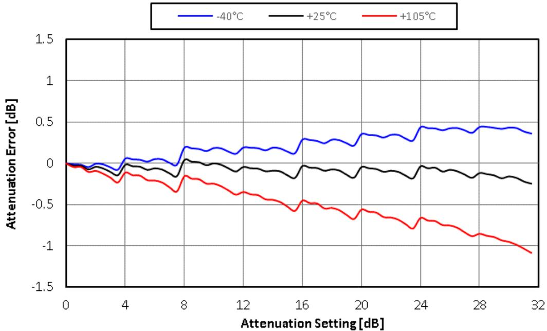
Figure 15. Attenuation Error @1800MHz vs Temperature
