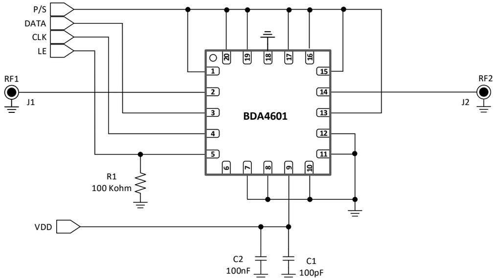
**Note:** 1. C1 and C2 should be placed near the device.
