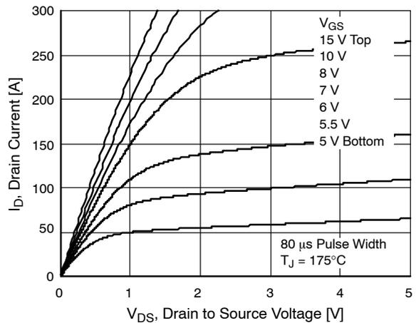
Figure 10. Saturation Characteristics
