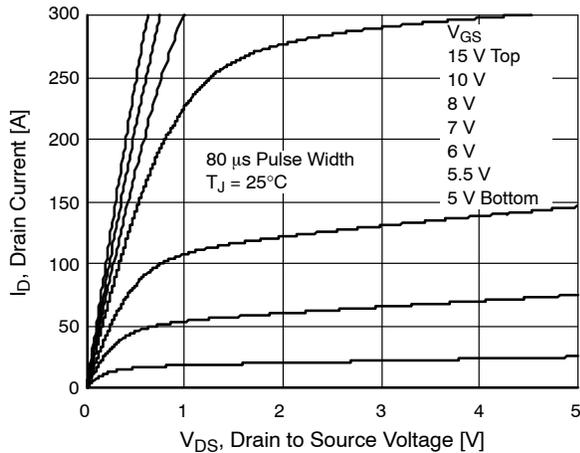
Figure 9. Saturation Characteristics
