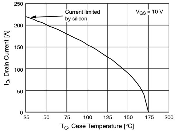
Figure 2. Maximum Continuous Drain Current vs. Case Temperature
