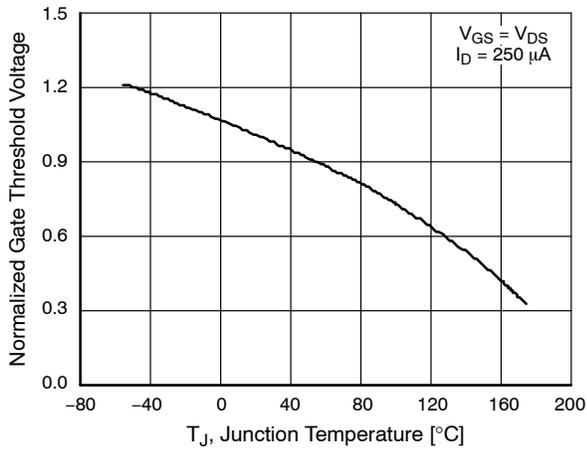
Figure 13. Normalized Gate Threshold Voltage vs. Temperature
