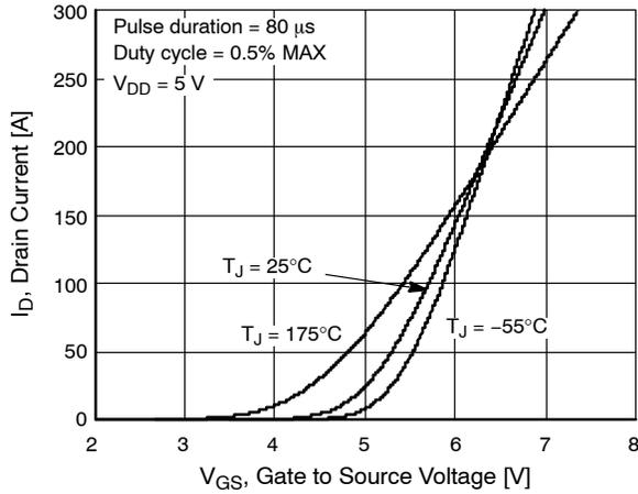
Figure 7. Transfer Characteristics
