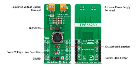
Buck-Boost 4 Click uses a standard 2-wire I2C interface to communicate with the host MCU supporting clock frequency of up to 1MHz. The I2C address can be selected over the ADDR SEL jumper. You can turn off the device by setting the EN pin to a LOW logic state. The fault indication is available over the INT pin.
