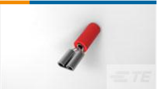
TE Part #640917-2 RECEPT,PIDG FASTON 22-18 187
