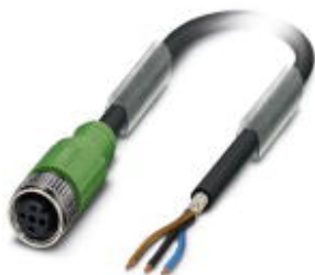
Sensor/actuator cable, 3-position, PUR halogen-free, black-gray RAL 7021, shielded, free cable end, on Socket straight M12, A-coded, cable length: 20 m
