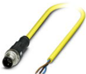
Sensor/actuator cable, 3-position, PVC, yellow, Plug straight M12 SPEEDCON, A-coded, on free cable end, cable length: 2 m
