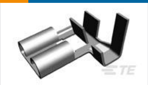
TE Part #63963-1 250 FASTON FLAG REC 18-14 AWG NPST
