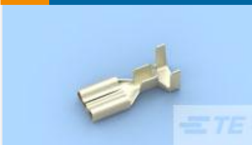
TE Part #1742899-1 187 FASTON,REC.,18-16 OR 2X18 AWG,NPST
