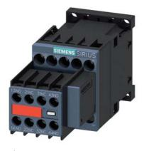
power contactor, AC-3e/AC-3, 9 A, 4 kW / 400 V, 3-pole, 230 V AC, 50/60 Hz, with varistor plugged on, auxiliary contacts: 2 NO + 2 NC, screw terminal, size: S00, captive auxiliary switch
