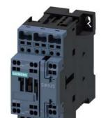
traction contactor, AC-3e/AC-3, 25 A, 11 kW / 400 V, 3-pole, 24 V DC, 0.7-1.25\* Us, electronic drive, with integrated varistor, auxiliary contacts: 1 NO + 1 NC, spring-loaded terminal, size: S0
