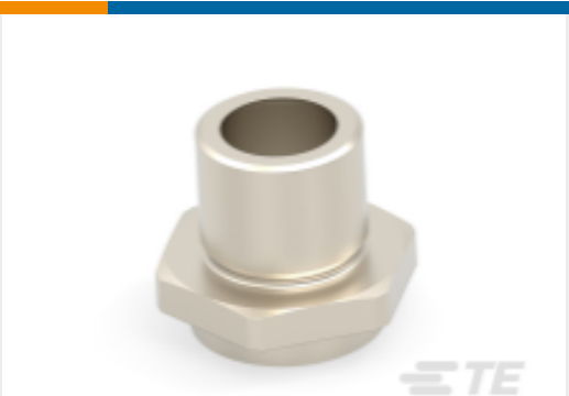
TE Part #284377-E M12 METAL SHELL, MALE, VERT, 13MM, D8.35
