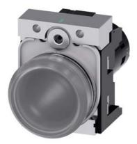
Indicator light with LED lamp, compact, 22 mm, round, metal, clear with red-yellow-green LED, lens, smooth, with holder, operating voltage 6-24 V AC/DC, screw terminal
