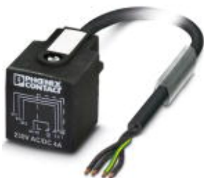
Sensor/actuator cable, 4-position, PUR halogen-free, black-gray RAL 7021, free cable end, on Valve connector AD (pressure switch), cable length: 3 m, Pin connector pattern of valve plug rotated 180°
