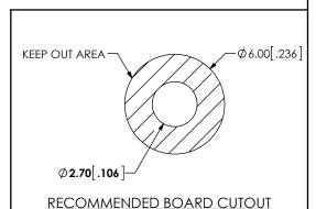
UNLESS OTHERWISE SPECIFIED, DIMENSIONS ARE IN MILLIMETERS TOLERANCES ARE: **DECIMALS ANGLES**
