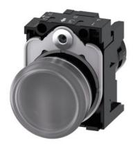
Indicator light with LED lamp, compact, 22 mm, round, plastic, clear with redyellow-green LED, lens, smooth, with holder, operating voltage 6-24 V AC/DC, screw terminal
