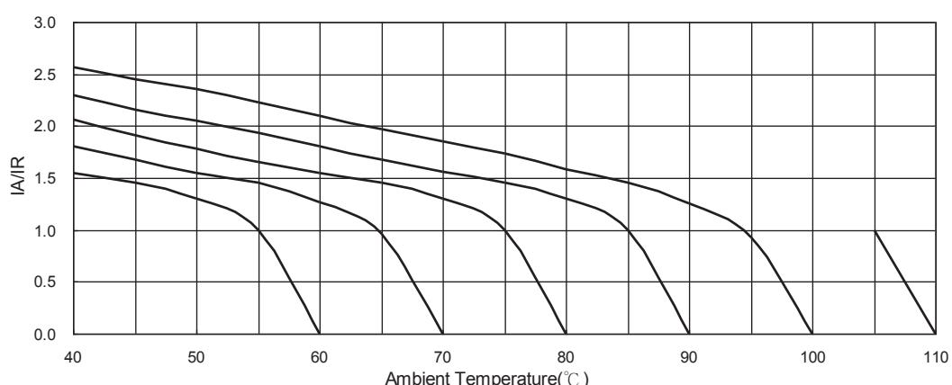
IA: Actual Ripple Current    IR: Rated Ripple Current
