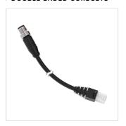
Cordset: Double Ended M12 to RJ45 8-pin Straight Male; 8-pin Straight Male 4.57 m 8x24 Shielded Black PVC Jacket Nickel-Plated Brass Coupling Nuts Part Number: 800008
