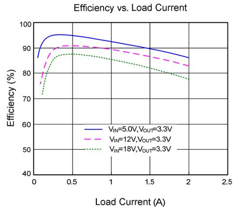
Figure 2. Efficiency Figure
