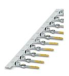
Crimp contact, Pin, rolled, Taped product, number of pieces per reel: 500, contact diameter: 1 mm, crimp range: 0.08 mm<sup>2</sup> ... 0.22 mm<sup>2</sup>
