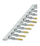
Crimp contact, Pin, rolled, Taped product, number of pieces per reel: 10000, contact diameter: 1 mm, crimp range:  $0.22~\text{mm}^2$  ...  $0.56~\text{mm}^2$ , Item is lead-free in accordance with RoHS II without Exemption 6c (Pb < 0.1~%)
