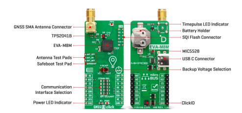
GNSS 11 Click can use the SPI, I2C, or UART interface to communicate with the host MCU, which can be selected over the five COMM SEL jumpers. By default, UART and I2C are selected. The I2C is actually a DDC interface (I2C compliant) and can be operated in slave mode only, supporting a clock frequency of up to 400kHz. If you choose an SPI interface, you can count on 125kbps and 5.5MHz of clock frequency.
