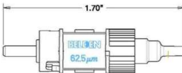
900 \mu\text{m} VERSION (OM1 SHOWN)
