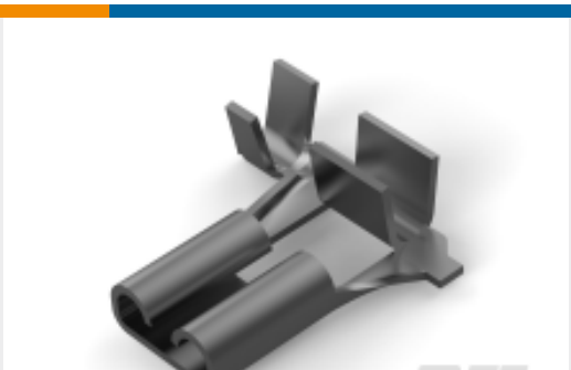
TE Part #1742685-1 FASTON 187 TERMINAL-FLAG REC 18 AWG TPBR
