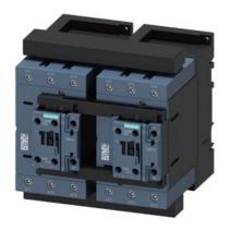
Reversing contactor assembly, AC-3, 45 kW 400 V, 230 V AC/50/60 Hz 3-pole, Size S3 screw terminal electrical and mechanical interlock 2 NO integrated
