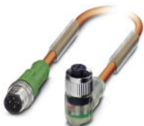
Sensor/actuator cable, 4-position, PUR halogen-free, irradiated, orange RAL 2003, Plug straight M12, A-coded, on Socket angled M12, A-coded, with 2 LEDs, cable length: 0.6 m, Customer-specific version
