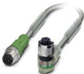
Sensor/actuator cable, 4-position, PUR halogen-free, highly flexible, gray RAL 7001, Plug straight M12, A-coded, on Socket angled M12, A-coded, with 3 LEDs, cable length: 0.3 m
