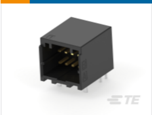
TE Part #1-2040516-5 Header Assembly: Wire-to-Board, 3A, Gold or Tin Plated
