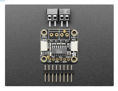
Each breakout comes with a NAU7802 ADC chip, plus some support circuitry, and 4 terminal blocks that can be used to connect a 4-wire sensor.
