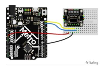
Board 5V to ADC VIN (red wire)
