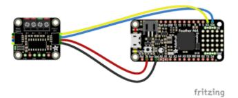
Board 3V to ADC VIN (red wire)
