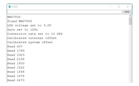
Attach a strain gauge with four wires to the four terminal inputs on the NAU7802. Upload the sketch to your board and open up the Serial Monitor (Tools -> Serial Monitor) at 115200 baud. You should see the values from the ADC being printed out. You'll see the value increase or decrease depending on the amount of force you are applying to the strain gauge.
