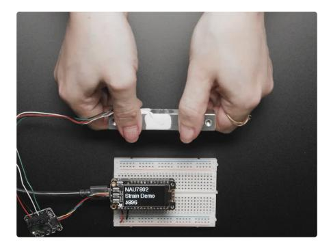
If you are feeling the stress and strain of modern life a Wheatstone bridge and you want to quantify it, this handy breakout will do the job, no sweat! The Adafruit NAU7802 contains a super-high-resolution 24-Bit differential ADC with extra gain and calibration circuitry that makes it perfect for measuring strain gauges / load cells or other sensors that have four wires that are connected in a Wheatstone bridge arrangement (https://adafru.it/-kd).
