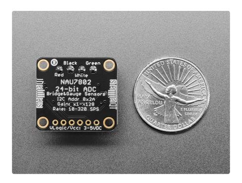
The E- pad connects to ground (often a black wire), the E+ pad connects to a generated voltage from the NAU7802 that can be configured from 2.4V to 4.0V for a solid positive reference (often a red wire).
