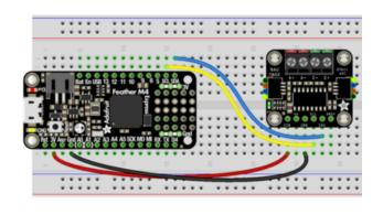
Board 3V to ADC VIN (red wire)
