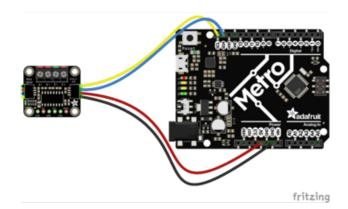
Board 5V to ADC VIN (red wire)
