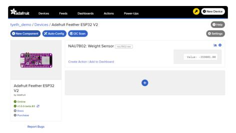
To view the data that has been logged from the sensor, click on the graph next to the sensor name.
