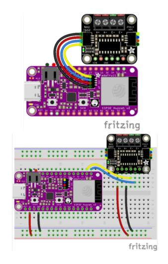
Board 3V to sensor VIN (red wire on STEMMA QT) Board GND to sensor GND (black wire on STEMMA QT)
