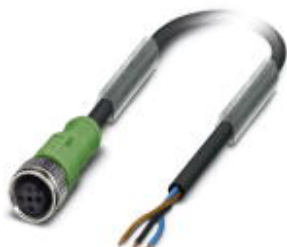
Sensor/actuator cable, 4-position, PVC, black RAL 9005, free cable end, on Socket straight M12, A-coded, cable length: 25 m
