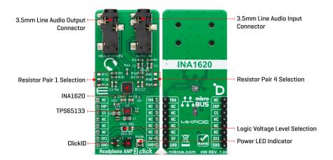
The INA1620 has two functional modes: a Shutdown and an Enabled mode. In Shutdown mode, the INA1620 will have minimal power consumption. However, applying signals to the output while in Shutdown mode will parasitically power the output stage of the audio amplifier. While in Enabled mode, the INA1620 uses a few tricks to clean things up. The INA1620 uses efficient electromagnetic interference (EMI) rejection as an immunity to change in offset, thus having a higher EMIRR.
