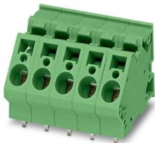
PCB terminal block, nominal current: 32 A, rated voltage (III/2): 630 V, nominal cross section: 4 mm<sup>2</sup>, number of potentials: 12, number of rows: 1, number of positions per row: 12, product range: ZFKDS(A) 4, pitch: 7.5 mm, connection method: Spring-cage connection, mounting: Wave soldering, conductor/PCB connection direction: 45 °, color: green, Pin layout: Linear pinning, Solder pin [P]: 3.5 mm, number of solder pins per potential: 2, type of packaging: packed in cardboard
