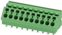
PCB terminal block, nominal current: 32 A, rated voltage (III/2): 630 V, nominal cross section: 4 mm<sup>2</sup>, number of potentials: 10, number of rows: 1, number of positions per row: 10, product range: ZFKDS(A) 4, pitch: 7.5 mm, connection method: Spring-cage connection, mounting: Wave soldering, conductor/PCB connection direction: 45 °, color: green, Pin layout: Linear pinning, Solder pin [P]: 3.5 mm, number of solder pins per potential: 2, type of packaging: packed in cardboard
