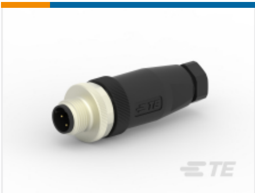
TE Part #T4111501041-000 M12,MALE,STRAIGHT,D CODE,4P, PG7,GOLD
