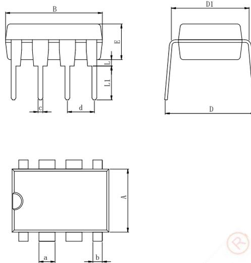
**Dimensions In Millimeters(DIP8L)**
