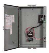
Pump control panel, Size 3 1/2, Three phase full voltage, Solid-state overload relay, OLR amp range 50-200A, 190-220/220-240V 50/60Hz coil, Standard type contactor, 125A circuit breaker, HOA Sel Sw. <(>&<)> Start P.B., Enclosure NEMA type 3/3R, Weather proof outdoor use
