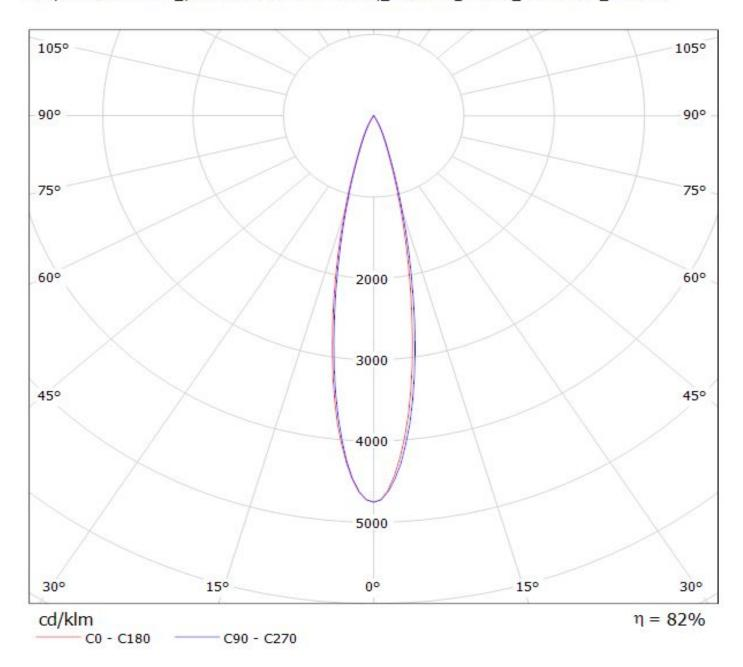
Luminaire: Ledil FC14970\_FLORENTINA-2X2-SS\_(Luxeon\_MZ) Lamps: 1 x Luxeon\_MZ\_2x2\_(LM29-SW30)\_1110.46Im@250mA\_P=11.0448W\_I=0.25A
