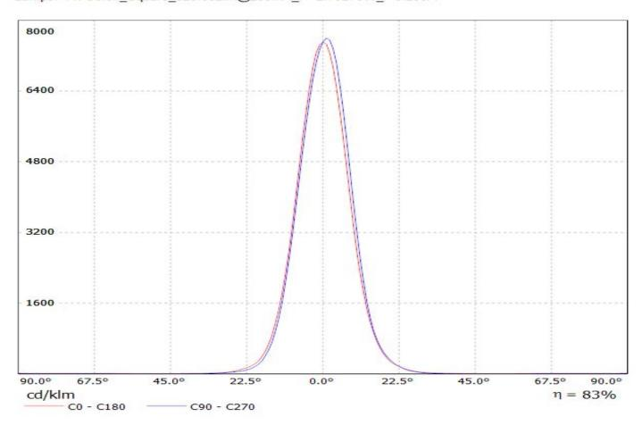
Luminaire: Ledil FC14970\_FLORENTINA-2X2-SS\_(SQ\_Gen3) Lamps: 1 x Oslon\_square\_GEN3\_(GW\_CSSRM2.PM-MUNQ-A737-1) \_453.421Im@250mA\_P=2.7755W\_I=0.25A
