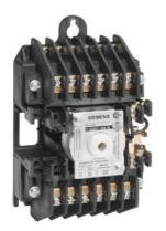
Mechanically held lighting contactor, Contactor amp rating 20Amp 0NC  $\_$  3NO poles, 265-277V 50/60HZ coil, Non-combination type, Enclosure NEMA type open, No enclosure
