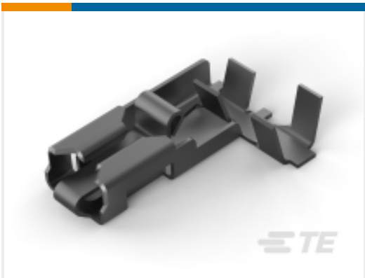
TE Part #965972-1 PL 250 REC TERMINAL-FLAG 17-13 PTPB
