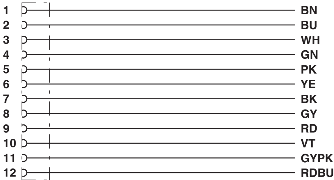
Contact assignment of the M12 socket
