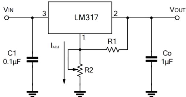
$$V_{OUT} = 1.25V \times (1 + R_2/R_1) + I_{ADJ} \times R_2$$
